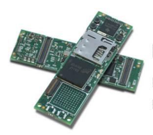
Processor: OMAP 3503 Application Processor with ARM Cortex-A8 CPU
